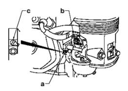
**Note:** On some engines, the pilot screw is fitted with a limiter cap (c) to prevent excessive enrichment of the air-fuel mixture in order to comply with emission regulations. The mixture is set at the factory and no adjustment should be necessary. Do not attempt to remove the limiter cap. The limiter cap cannot be removed without breaking the pilot screw.
